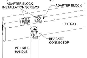
2.A. GLASS MOUNT HANDLE. Insert rubber bushing into glass hole at top of glass door. Place exterior pivot bracket against exterior side into notched portion of glass. Align interior handle with exterior pivot bracket and tighten low head cap screw. Check the alignment and gentle remove the interior handle. Tighten 1/4-20 set cap screws. Install handle and start thread at bottom pivot end.
