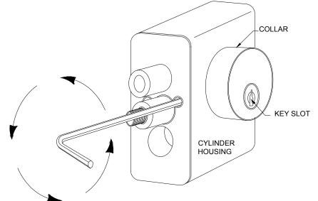
Remove old cylinder and check to see if tailpiece matches new cylinder tailpiece. Also the length of the new cylinder must be the same as the old one. A cylinder of any other length will require a new length collar. Wind in new cylinder until it stops inside the collar ring.
