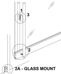
Push two #10-24 FHSS flush with housing and place the interior handle on the door over pivot end on the rail.
