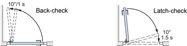
The back-check will be automatically adjusted to 10° and 1 second before open position. The latch-check will be automatically adjusted to 10° and 1.5 seconds before closed position.
