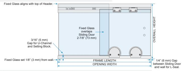
NOTE: Drawings not shown to scale. Frame is cut 1/16" (2 mm) less than Opening Width and centered in opening. Overall Height is height from curb/floor to top of Header. Drawings shown from interior.
