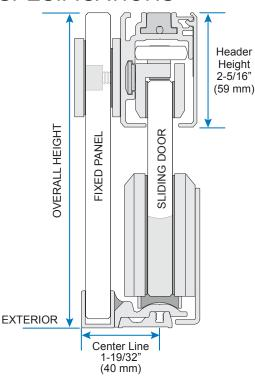
NOTE: For use with 3/8" or 1/2" (10 or 12 mm) Tempered Glass. Do Not use Laminated Glass.
