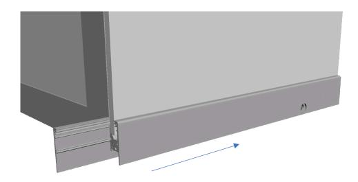
**STEP 3:** If a CRL 777S Rail Lock is being used, install the cylinder by tightening the cylinder set screws at the end of the Rail Body.
