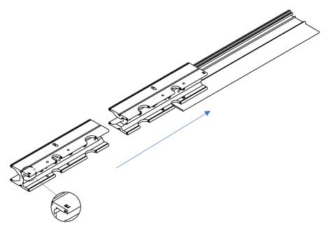
IMPORTANT: Each Rail Body is marked with an "E" on one end. On the pivot side Rail Body, the "E" must face out towards the glass edge.
