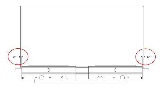
**STEP 5:** After proper positioning is achieved, pull the spacer blocks out from each of the Rail Bodies, then push the Rail Body clamps over the glass until the glass bottoms out on the nut strip.
