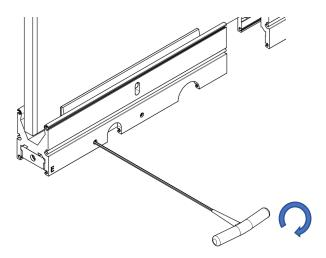
**STEP 3:** Tighten the Set Screw that was loosened (furthest from the pivot) until it touches the Adjustable Slide Block (you will feel resistance to tightening).
