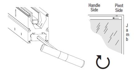
**Helpful Hint:** One full turn of the socket head cap screw will adjust the door 1/16" (1.6 mm)
