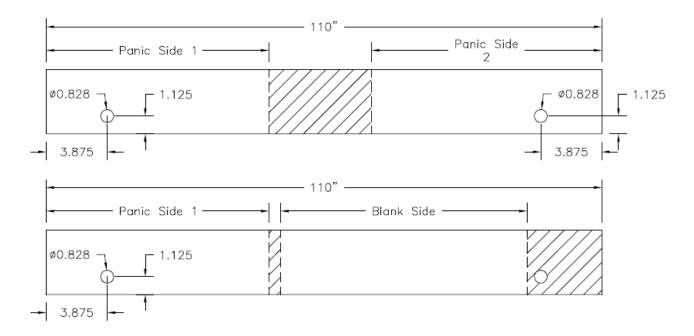
**NOTE:** If the glass door requires a Blumcraft $^{\circ}$  Panic/Egress/Deadbolt device, you will need the following hardware: CRL MPH53 Block with 5/16-18 socket head cap, Length = 1", installation screws (2). Included w/purchase of ACH device.
