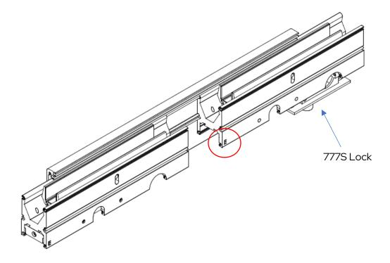
**STEP 3:** Slip Rail Bodies with Side Cover onto the glass.
