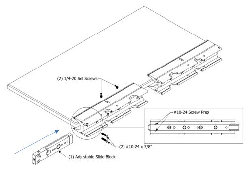
**Optional:** Install CRL 777S Lock on the swing side Rail Body. The Rail Body is pre-prepped for lock installation. Remember that for lock installation, the swing side Rail Body must be flipped so that the **"E"** is on the inside.
