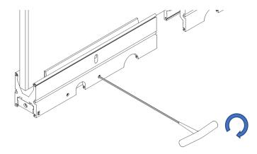
**STEP 3:** Tighten the Set Screw that was loosened (closest to the pivot) until it touches the Adjustable Slide Block (you will feel resistance to tightening).
