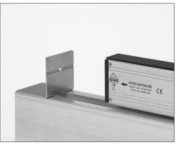
Laser light pinpoints on LT1 Laser Target.
