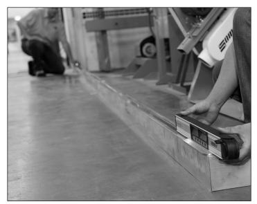
Align the "PAL" Tool with base shoe and point toward the Laser Target set at other end of Base Shoe.
