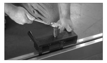
Make sure the blade movement mechanism of the TLK5 Tool moves freely, and hasn't become filled with dust or debris. Blade mechanisms that are poorly maintained may cause binding during the Taper compression operation, and result in an improper installation with insufficient compression of the Tapers.
