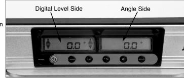
Display for Digital Level and Angle Locator.
