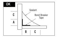
(1) Dimension A, B, and C must be at least 1/4" (6 mm); (2) A bond breaker tape or backer rod must be present if joint movement is anticipated; (3) Joint must be tooled into a concave surface; (4) Minimum sealant thickness of 1/8" (3 mm).
