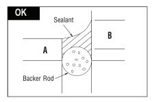
(1) Dimensions A and B are both greater than 1/4" (6 mm); (2) Sealant tooled to ensure positive runoff of water.
