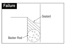
(1) Water could accumulate on top of the improperly tooled joint. increasing the chance of "pooling" and the probability of joint failure.
