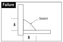
(1) Dimension A or B less than 1/4" (6 mm); (2) Joint not properly tooled into a concave surface; (3) No bond breaker material; therefore the joint will not accept movement.
