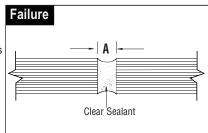
(1) Dimension A less than 1/4" (6 mm) resulting in inconsistent joint fill and very limited movement capabilities; (2) Clear sealants susceptible to yellowing from window cleaning chemicals, intersecting organic gaskets, and tobacco smoke; shows glass defects and bubbles.
