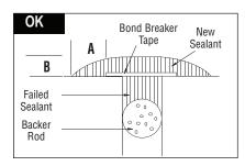
(1) Dimension A must be at least 1/4" (6 mm): (2) Dimension B must be at least 1/8" (3 mm) to a 3/8" (9.5 mm) maximum; (3) Bond breaker tape must be used to isolate fresh sealant from failed sealant.
