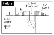
(1) Dimension A less than 1/4" (6 mm): difficulty in obtaining adhesion and increases the likelihood for gaps; (2) Dimension B less than 1/8" (3 mm): increases the likelihood of pinholes or voids in tooling; poor cohesive integrity. (3) No bond breaker tape: increases the chance that the sealant will tear when the underlying substrates move.
