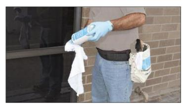
The Correct method is to pour on the cleaner. Dipping the rag into the solvent is incorrect, as this will contaminate the cleaning agent.
