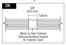
(1) Minimum 1/4" (6 mm) joint width; (2) Minimum 1/4" (6 mm) glass thickness; (3) Joint tooled into hourglass shape; (4) Dark-colored silicone building sealant is recommended (exterior).
