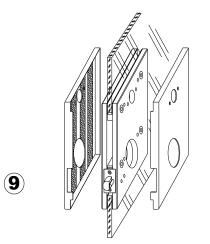
REMOVE VHB TAPE COVER PAPER CAREFULLY APPLY COVER PLATES ENSURING HOLES AND LOCK FACE PLATE LINE UP. PRESS ON FIRMLY.
