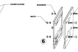
SEPARATE CLAMP PLATES BY REMOVING 4 CAP HEAD SCREWS NUTS AND WASHERS.
