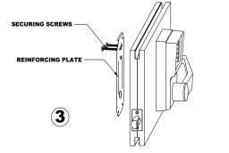
REMOVE REINFORCING PLATE BY UNSCREWING THE TWO SECURING SCREWS
