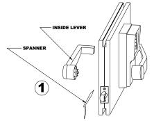
REMOVE INSIDE LEVER BY INSERTING POINT OF SPANNER INTO POKEHOLE IN COLLAR OF DRIVE SLEEVE AND DEPRESSING RETAINING CLIP.
