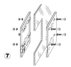
ASSEMBLE CLAMP PLATES ONTO GLASS. BE SURE TO HAVE NUTS AND WASHERS ON THE OUTSIDE
