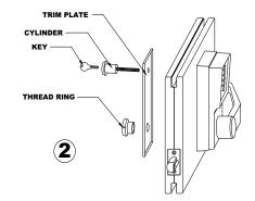
REMOVE CYLINDER BY INSERTING KEY AND ROTATING CYLINDER ANTI-CLOCKWISE UNTIL IT IS FREE.
