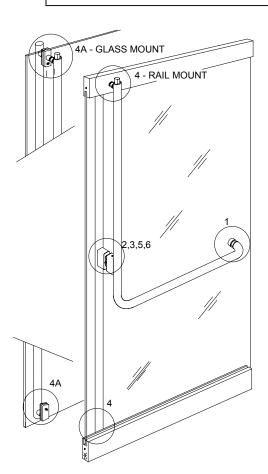
Insert rubber bushings into glass holes for exterior retainer cap. Place the retainer in position on exterior side of glass and tighten retainer cap through rubber bushing. Install stud with locking nut through washer w/gasket and tighten.
