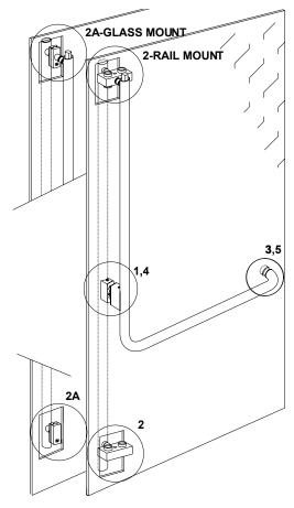
1. To remove the Handle from the board first loosen two flat head socket screws (A) they protrude so
