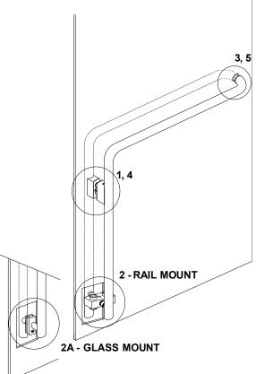
To remove the Handle from the board first loosen two flat head socket screws
