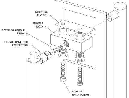
2.A. FOR GLASS MOUNT HANDLE. Remove Socket Head Cap Screw from Interior Pivot Bracket and Exterior Bracket. Be careful not to lose Gaskets located between Interior and Exterior Brackets
