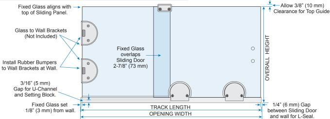
NOTE: Drawings not shown to scale. Track is cut 1/16" (2 mm) less than Opening Width and centered in opening. Overall Height is height from curb/floor to top of glass. Drawings shown from interior.
