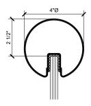
GR40 CAP RAIL 4" DIAMETER FOR 1/2" TO 5/8" GLASS STAINLESS STEEL
