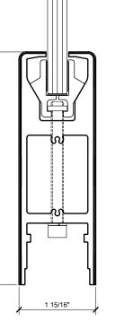
DR6SPS12S - POLISHED STAINLESS DR6SBS12S - BRUSHED STAINLESS >MATERIAL: ALUM. >FINISH: MILL >CLAD: YES >CLAD MATERIAL: 20GA (.035") STAINLESS STEEL >GLASS: 1/2", TEMPERED, MONOLITHIC
