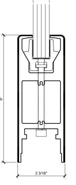
DR6SPS34S - POLISHED STAINLESS DR6SBS34S - BRUSHED STAINLESS DR6SPS58S - POLISHED STAINLESS DR65B558S - BRUSHED STAINLESS >MATERIAL: ALUM. >FINISH: MILL >CLAD: YES >CLAD MATERIAL: 20GA (.035") STAINLESS STEEL >GLASS: 5/8" & 3/4", TEMPERED, MONOLITHIC
