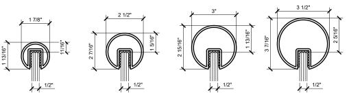
GR35M CAP RAIL 1/2" TO 5/8" TEMPERED MONOLITHIC GLASS SET W/ GR5PV CAP RAIL RIGID VINYL INSERT
