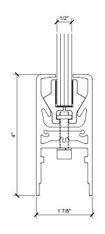
DR4SSA12S - SATIN ANODIZED DR4SDU12S - DARK BRONZE ANODIZED DR4SBL12S - BLACK POWDER COAT >MATERIAL: ALUM. >CLAD: NO >GLASS: 1/2", TEMPERED, MONOLITHIC
