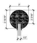
WCR30 CAP RAIL 3" DIAMETER FOR 1/2" TO 5/8" GLASS WOOD
