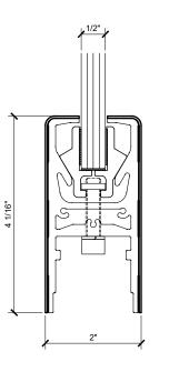
DR4SPB12S - POLISHED BRASS DR4SSB12C - SATIN BRASS >MATERIAL: ALUM. >FINISH: MILL >CLAD: YES >CLAD MATERIAL: .045" BRASS >GLASS: 1/2", TEMPERED, MONOLITHIC
