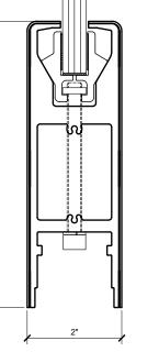
DR6SPB12S - POLISHED BRASS DR6SSB21C - SATIN BRASS >MATERIAL: ALUM. >FINISH: MILL >CLAD: YES >CLAD MATERIAL: .045" BRASS >GLASS: 1/2", TEMPERED, MONOLITHIC
