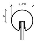
GR35 CAP RAIL 3-1/2" DIAMETER FOR 1/2" TO 5/8" GLASS STAINLESS STEEL
