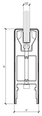
DR6SSA12S - SATIN ANODIZED DR6SSA12S - SATIN ANODIZED DR6SDU12S - DARK BRONZE ANODIZED DR6SBL12S - BLACK POWDER COAT >MATERIAL: ALUM. >FINISH: MILL >CLAD: YES >CLAD MATERIAL: .050" SHEET METAL >GLASS: 1/2", TEMPERED, MONOLITHIC
