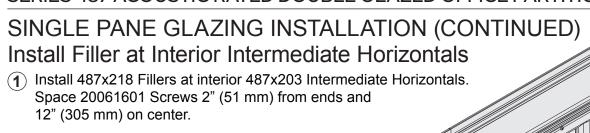
NOTE: Adjust screw spacing to avoid Clips. See placement chart below.
