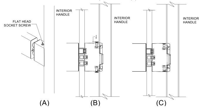
2. FOR RAIL MOUNT HANDLE. Rotate round connector pivot fitting counter clockwise and remove from Adapter Block. Note: Use pliers and rubber strip (to protect finish) for removal of round connector. Remove the Exterior Handle Screw to release the exterior handle from the adapter block.
