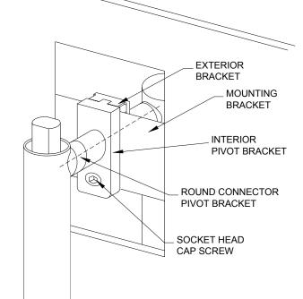
3. Remove two cap screws from the inside of the Cylinder Housing, and remove the housing from the board. Support and remove exterior cylinder housing, rubber bushings and spacer
