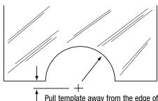
Pull template away from the edge of the glass—equal to the thickness of the channel bottom
