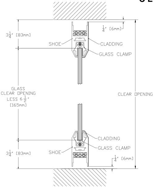
4" TAPERED DOOR RAIL TOP AND BOTTOM CLAD OR NON CLAD
