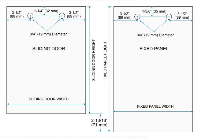
SLIDING DOOR AND FIXED PANEL WIDTH: Overall Width Divided by 2, plus 7/8" (22 mm)
