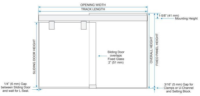
NOTE: Drawings not shown to scale. Track is cut 1/16" (1.5 mm) less than Opening Width and centered in opening. Overall Height is height from curb/floor to top of fixed glass. Drawings shown from interior.
