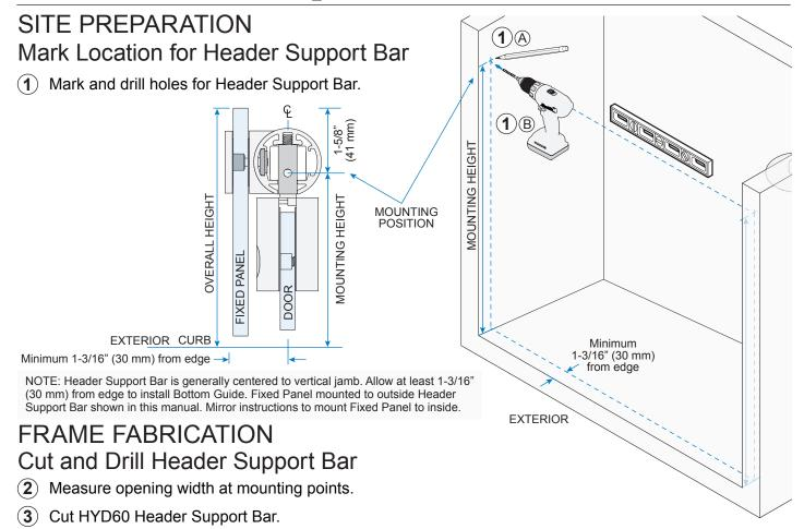
NOTE: Header Support Bar is cut 1/16" (1.5 mm) short from tight dimension and centered in opening, leaving 1/32" (.8 mm) gap on each end to mount. Refer to Fixed Panel Glass fabrication and gap allowance between Fixed Panel and wall to determine mounting hole placement.
