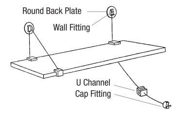
3. Hang Shelf: Put U-Channels on back and front of shelf as shown, drop Cap Fitting onto Wall Fitting (make sure they are properly aligned and fitted). Level shelf (front to back) by pulling Cable from below and pushing the shelf down into place.
