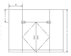
Figure 20. Interior Entrance Size when Supported at Head and Sill
