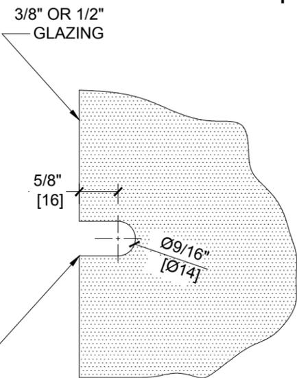
(1) FABRICATION SLOT CUTOUT IS REQUIRED WHEN USING THE PROVIDED STEEL PIN
