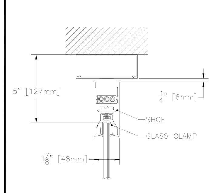
4" SQUARE DOOR RAIL UNCLAD WITH UNCLAD HEADER
