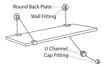
**3. Hang Shelf:** Put U-Channels on back and front of shelf as shown, drop Cap Fitting onto Wall Fitting (make sure they are properly aligned and fitted). Level shelf (front to back) by pulling Cable from below and pushing the shelf down into place.
