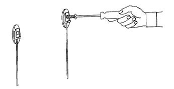
1. Choose Locations of Brackets: Preferably on wall studs, and make level marks for screws. 40" (1016 mm) is the maximum span between Brackets.
