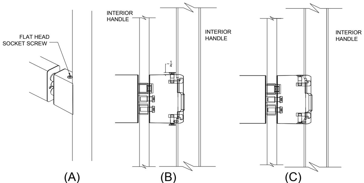
2. FOR RAIL MOUNT HANDLE. Rotate round connector pivot fitting counter clockwise and remove from Adapter Block. Note: Use pliers and rubber strip (to protect finish) for removal of round connector. Remove the Exterior Handle Screw to release the exterior handle from the adapter block.
