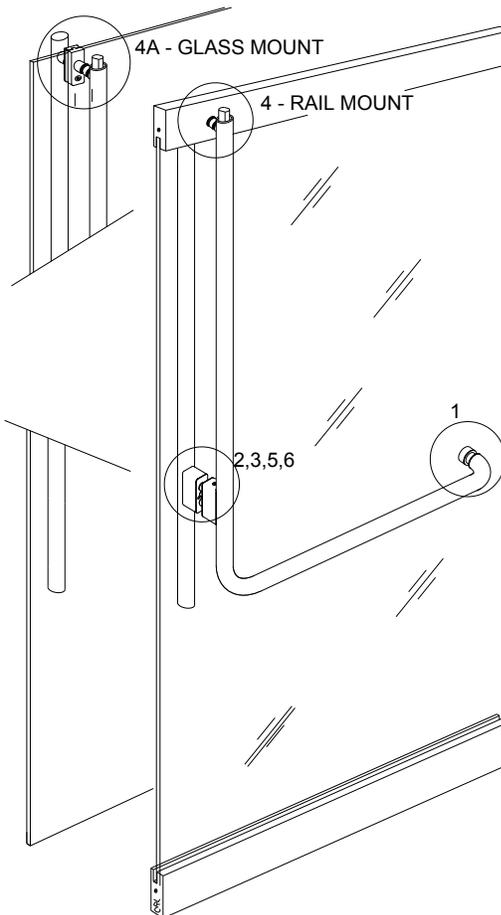
1. Insert rubber bushings into glass holes for exterior retainer cap. Place the retainer in position on exterior side of glass and tighten retainer cap through rubber bushing.
