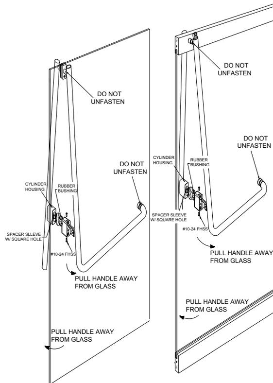
1. Loosen the flat head cap screws for approximately 1/8".
