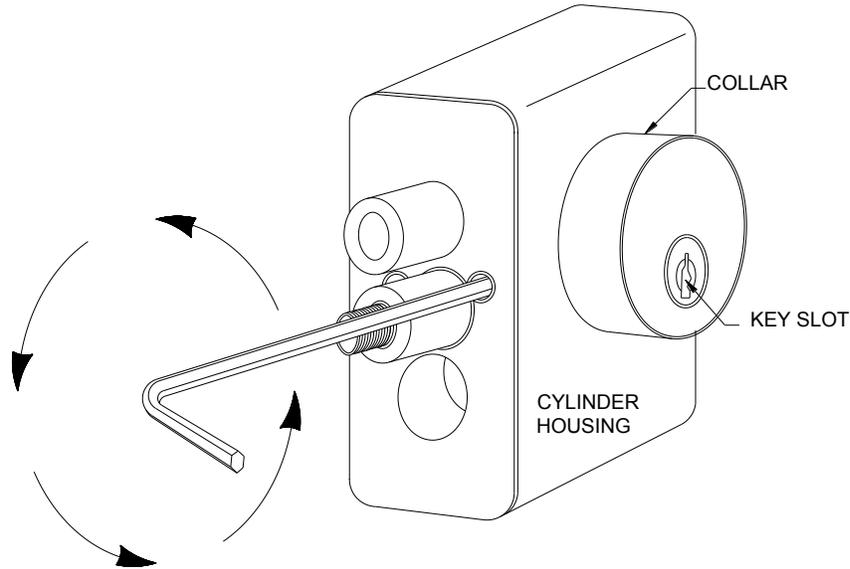
7. Remove old cylinder and check to see if tailpiece matches new cylinder tailpiece. Also the length of the new cylinder must be the same as the old one. A cylinder of any other length will require a new length collar. Wind in new cylinder until it stops inside the collar ring. Key slot should be on bottom of cylinder nearest the floor.
