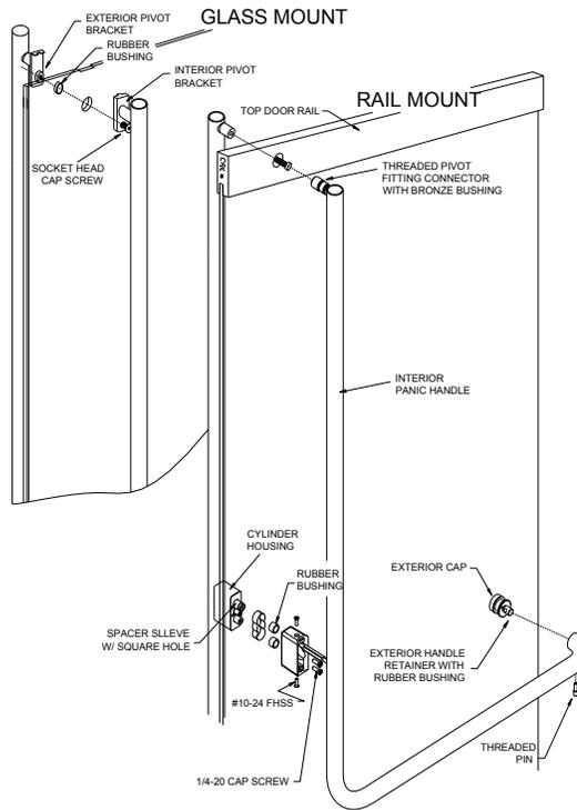
2. Install exterior lock housing with rubber bushing and spacer sleeve being careful that the square hole is facing the exterior handle with sides of hole in line with the handle width, and the lock cylinders in both housings are facing the hinge side of the doors. For installation of both housing together use two 1/4-20 cap screws. Finger tight.
