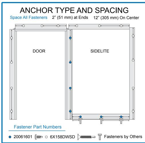
All vertical members are cut with an additional 1-5/8" (41.3 mm) Scribe length for field cutting to allow for varying unlevel floor conditions. Fabricated frames can be ordered to exact dimensions for "cut-free" installation.
