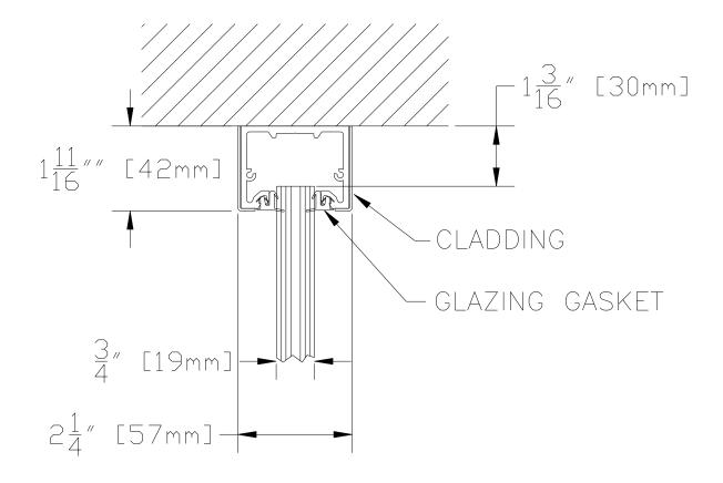
NARROW HEADER FOR 3/4" GLASS CLAD
