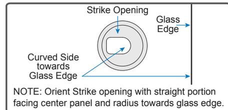
NOTE: Orient Strike opening with straight portion facing center panel and radius towards glass edge.
