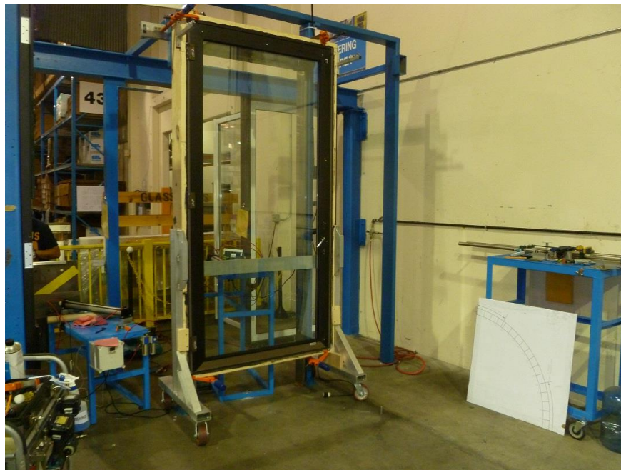
Photo No. 2 Door Cycling Set-Up – Exterior
