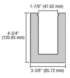
Shoe strength – Vertical legs: Glass reaction by bearing on legs to form couple. Allowable moment on legsper 2020 ADM Chapter F.  $M_a = 1.5SF_y/\Omega_y$  or  $\leq ZF_u/\Omega_r$   $S_y = 12"*0.75"^{2*}/6 = 1.125 \text{ in}^3/\text{ft}$   $Z_y = 12"*0.75"^{2*}/4 = 1.6875 \text{ in}^3/\text{ft}$   $M_{ay} = 16\text{ksi}*1.5*1.125 \text{ in}^3/\text{ft}/1.65 = 16,364\#''/\text{ft}$  or (controls)  $M_{ar} = 22\text{ksi}*1.6875 \text{ in}^3/\text{ft}/1.95 = 19,038\#''/\text{ft}$
