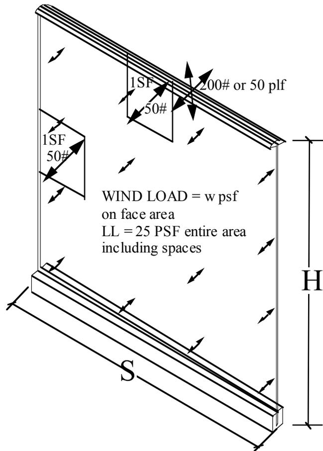
FOR WIND SCREEN OR DIVIDER APPLICATIONS WHERE FALL PROTECTION IS NOT REQUIRED THE CAP RAIL MAY BE OMITTED.
