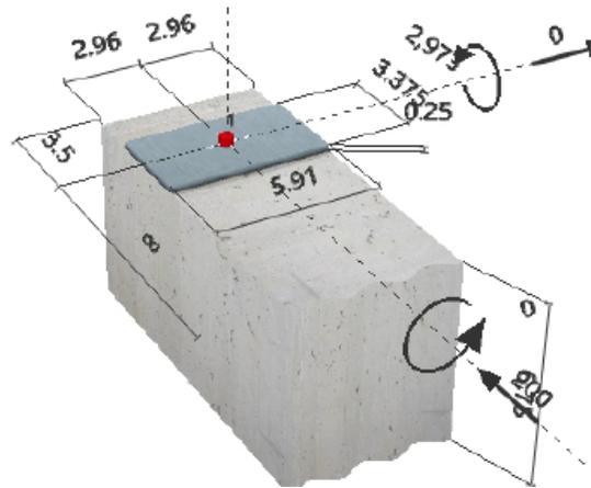
Shear load:  $V_u = 200\#$ ;  $V_a = 200/1.6 = 125\#$  per anchor
