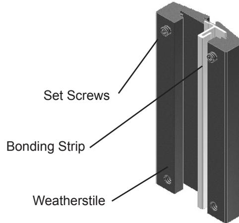
2. Slide both Cladding Strips over the Weatherstile but do not remove the tape liner. "Dry-Fit" the stile over the edge of the glass with the Bonding Strip below the glass to make sure the assembly fits between the top and bottom rails.
