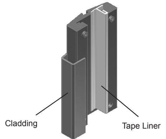
Pull the unit away and remove the Cladding Strips and the tape liner on the Bonding Strip. Press the assembly into place adhering it permanently into position against the glass surface.
