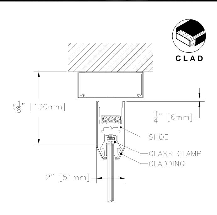
4" TAPERED DOOR RAIL CLAD WITH CLAD HEADER
