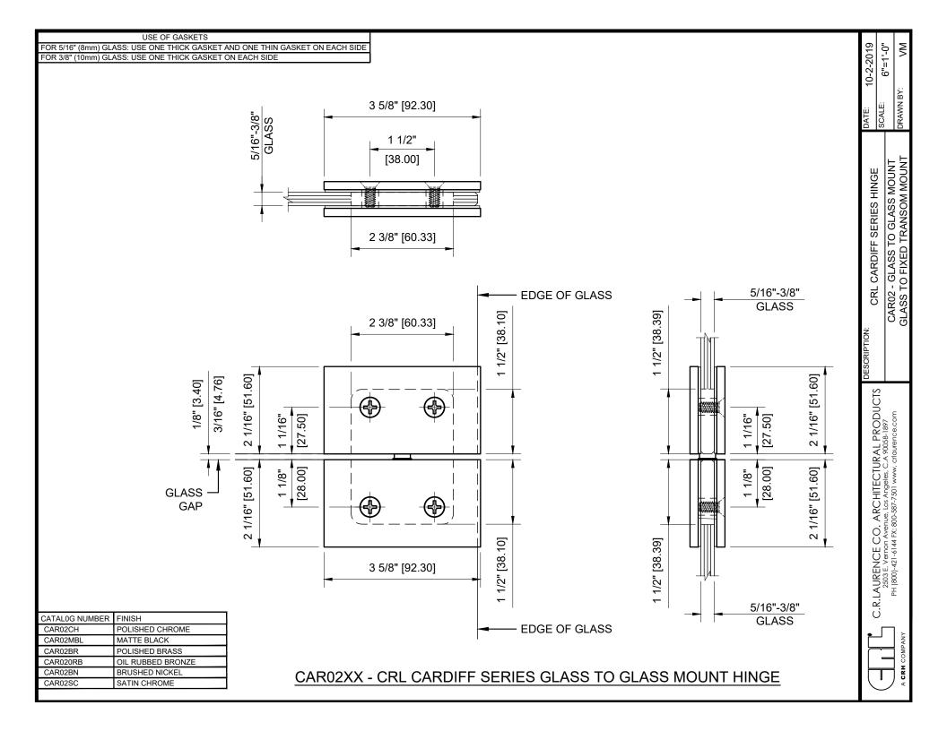
FOR 3/8" (10mm) GLASS: USE ONE THICK GASKET ON EACH SIDE
