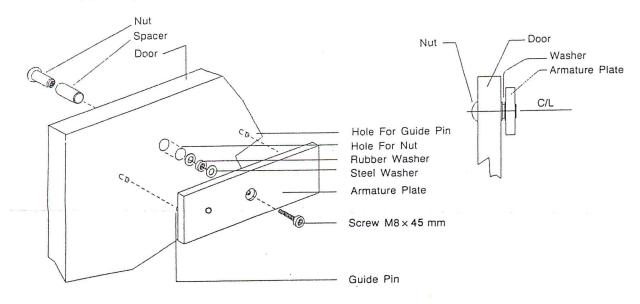
\*\* Important: Fix the armature plate not too tightly, and make the rubber washer more flexible, in order to make the armature plate automatically adjust its proper position with the magnet.
