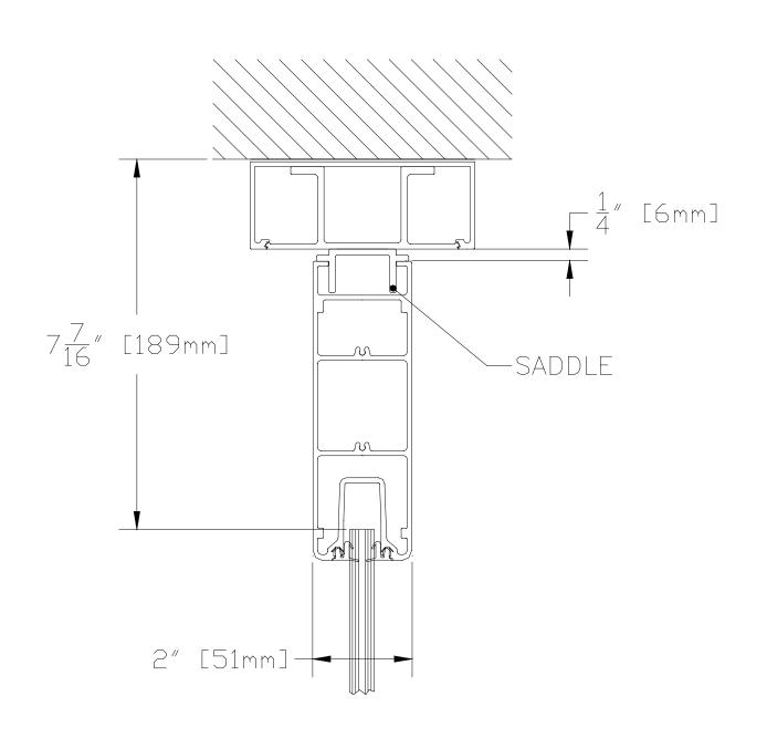
6" SQUARE SIDELITE RAIL UNCLAD WITH 1/4" SADDLE WITH UNCLAD HEADER
