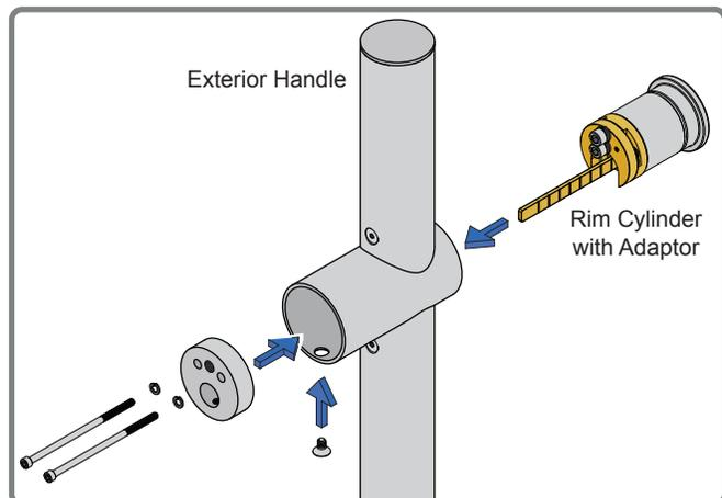
NOTE: Rim Cylinder may be substituted with Rim Cylinders with vertical tail pieces at least 2-1/2" (64 mm) long.
