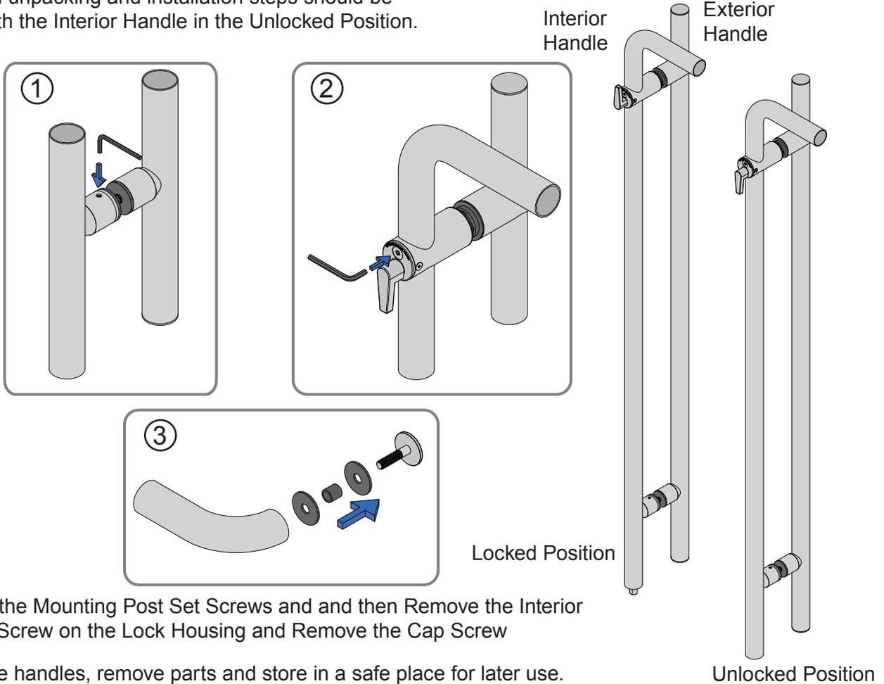
Loosen the Mounting Post Set Screws and then Remove the Interior Handle Screw on the Lock Housing and Remove the Cap Screw
