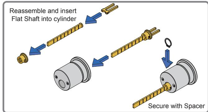
4. Install the Adaptor onto the new Rim Cylinder and reattach the new base and Cylinder to the Exterior Handle.
