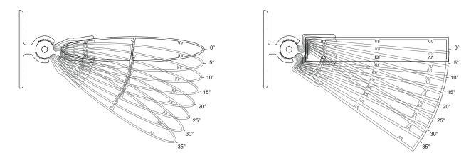
Blade angle can be customized by using the internal bracket grooves
