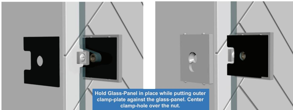
Hold Glass-Panel in place while putting outer clamp-plate against the glass-panel. Center clamp-hole over the nut.
