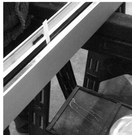
**NOTE:** All of the illustrations in this manual show the frame sill unmounted for clarity. Under actual conditions, the frame should be mounted and the screw heads sealed prior to installing the diffuser. The doors will be installed after the diffuser is in place.
