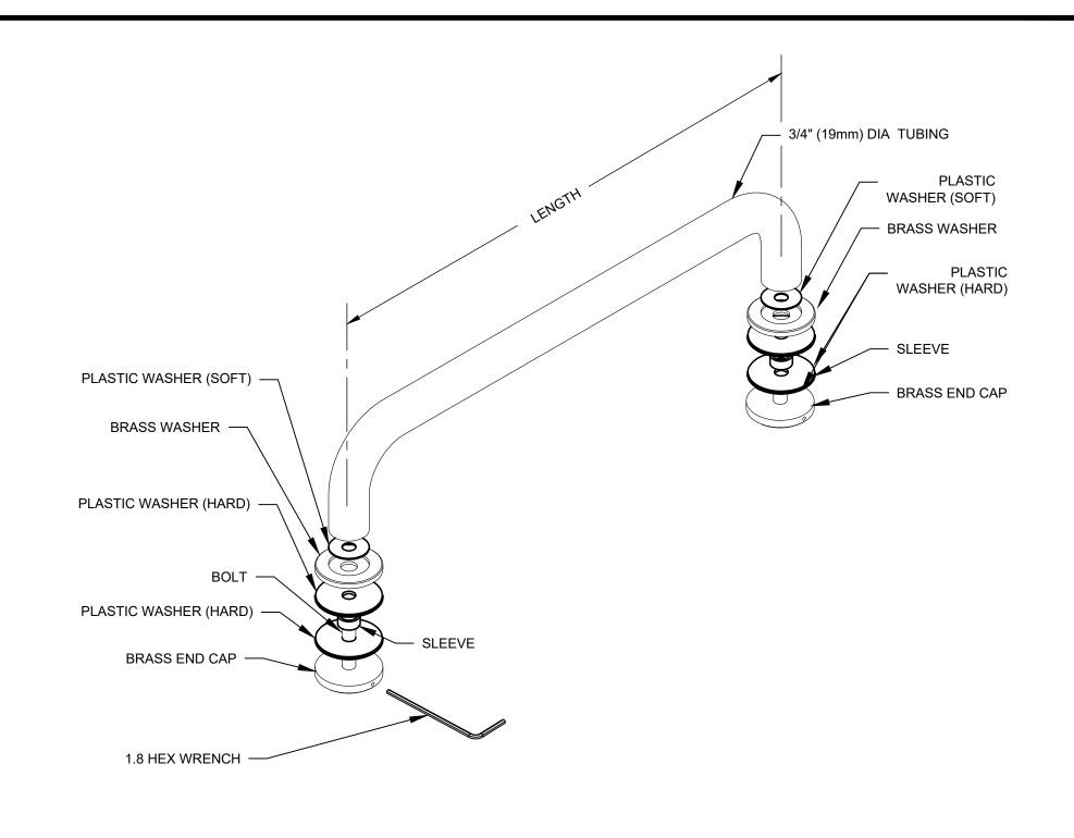
Material: 3/4" (19mm) dia. Brass Tubing .060" (2mm) thk. 1-1/4" (32mm) dia. metal washers Glass Thickness Range: 1/4" to 1/2" (10mm - 13mm) Hole Diameter Required: 1/2" (13mm)
