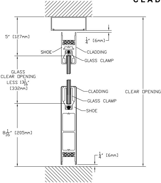
4" SQUARE DOOR RAIL TOP NON CLAD 10" SQUARE DOOR RAIL BOTTOM CLAD WITH NON CLAD HEADER
