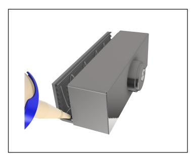
Apply CRL 95CBL silicone to lock body gaskets (Sides and Bottom).
