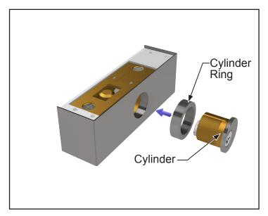
2. Install cylinder ring and cylinder (Cylinder lock **MUST** be in the horizontal position).
