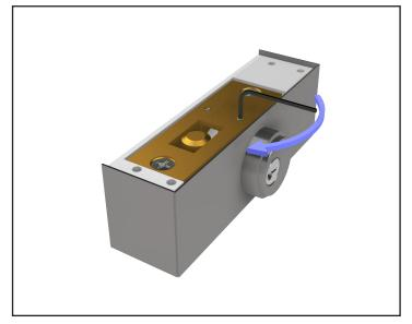
4. Secure cylinder in place by tightening the set screw.
