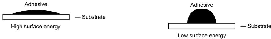
This illustration demonstrates the effect of surface energy on adhesive interfacial contact. High surface energy materials draw the adhesive closer for high bond strength.
