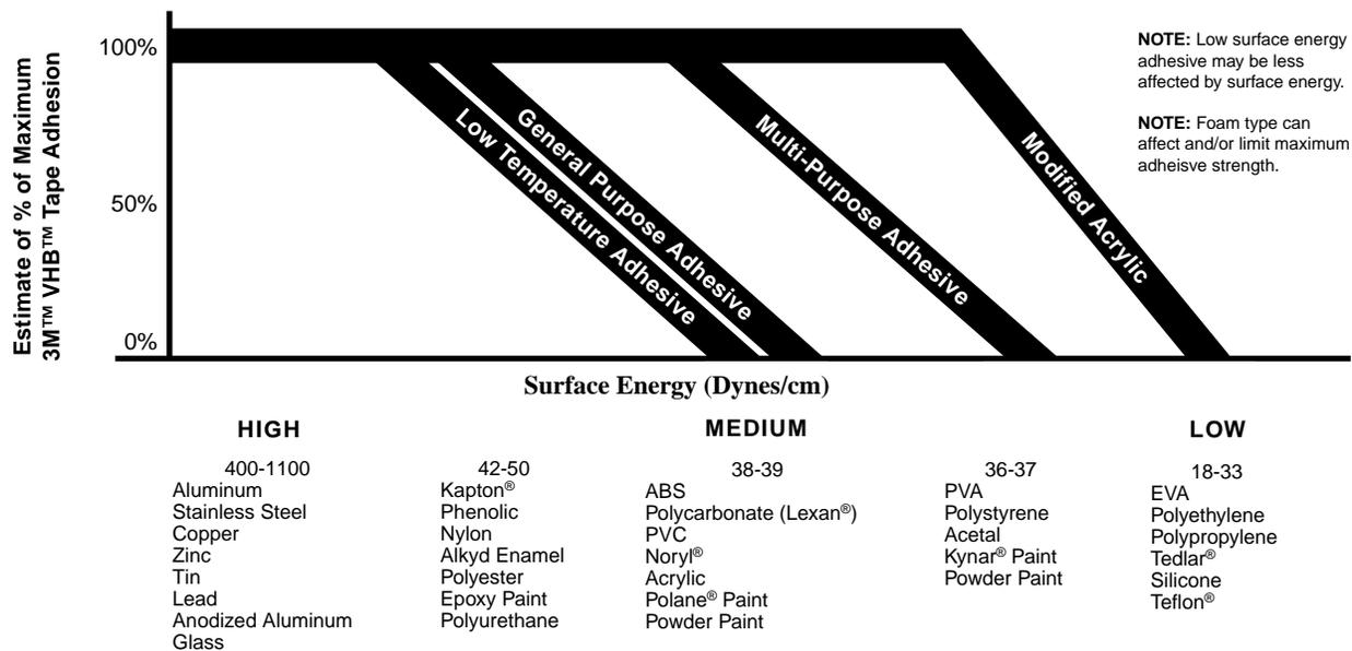
**NOTES:** There are a wide variety of formulations, surfaces finishes and surface treatments available on substrate materials which can affect adhesion. This chart is intended to provide only a rough estimate of the adhesion levels which can be expected on some common materials relative to a reference surface such as aluminum. Light surface abrasion will significantly increase adhesion levels on many materials, except when using tapes 4952/4932.
