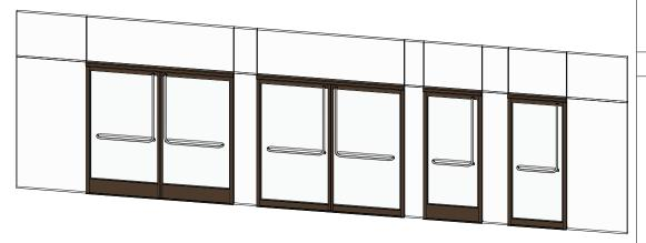
An unmistakable feature of Entice HP+ is its unique ability to support Blumcraft® Panic Devices and other types of handle hardware directly on dual-glazed 1" insulating glass units. This is achieved using precision-engineered, through-glass fittings. Despite the floating-onair aesthetic, panic devices pass the UL emergency exit load
