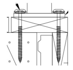
Typical installation will use 3/8"x6" SS lag screws: A typical installation is a 3/4" decking above solid blocking or beam that is protected from moisture, p = 6"-3/4"-7/32" = 5.03" W'p = 477pli\*5.03" = 2,400# > 1,940# greater than assumed minimum steel strength
