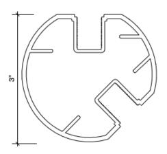
For balanced loading, loading in the Y-axis is zero and bending in the Z-axis is cos(22.5°) times the loading from each direction. Since the loading to the corner post is less than the loading to an intermediate post with the same spacing and the strength of the corner post is higher, it can be assumed in most cases that the corner post does not limit post spacing.
