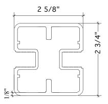
Allowable stress in aluminum post in accordance with ADM Design Aid Table 2-19: 6061-T6 Extruded aluminum
