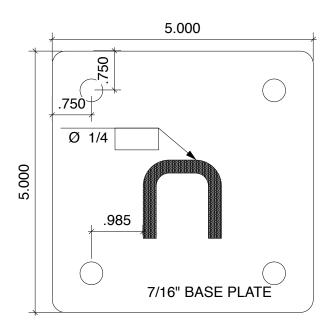
Maximum allowable moment on base plate:  $M_a = 2T_s^*(5"-0.75")$   $M_a = 2^*2,951\#*4.25" = 25,084"\#$ Base plate strength is adequate to develop the full stanchion plastic moment.
