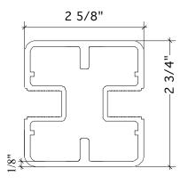
Allowable stress in aluminum post in accordance with ADM Design Aid Table 2-19: 6061-T6 Extruded aluminum Check local buckling of flat edge with intermediate stiffener: b/t = 2.1"/0.125" = 16.8 < 20.8 (Local buckling does not control)  $F_c/\Omega = 21.2ksi$  $M_a = 1.506in^{3*}21.2ksi = 31,900"\# = 2,660'\#$
