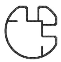
Allowable stress in aluminum post in accordance with the 2015 ADM Design Aid Table 2-19:  $R_b/t = 1.42$ "/0.079" = 18.0 < 27.6 not subject to local buckling
