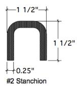
Material: HR Steel A1011, A572 Grade 50, or equal. Finish: Black Powder Coat
