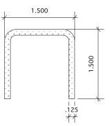
The stanchions are installed so that primary bending axis is YY with essentially no bending in the XX direction.
