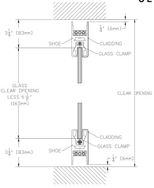
4" SQUARE DOOR RAIL TOP AND BOTTOM CLAD OR NON CLAD
