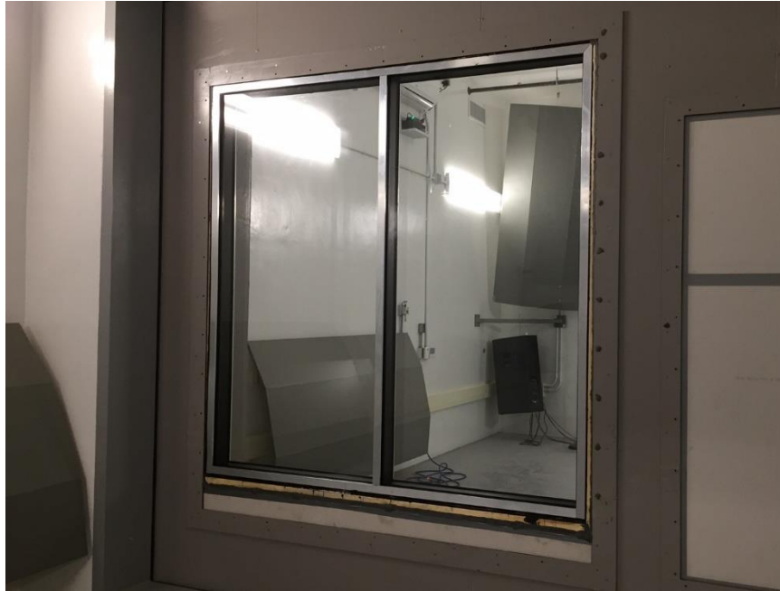
Receive Room View of Installed Specimen
