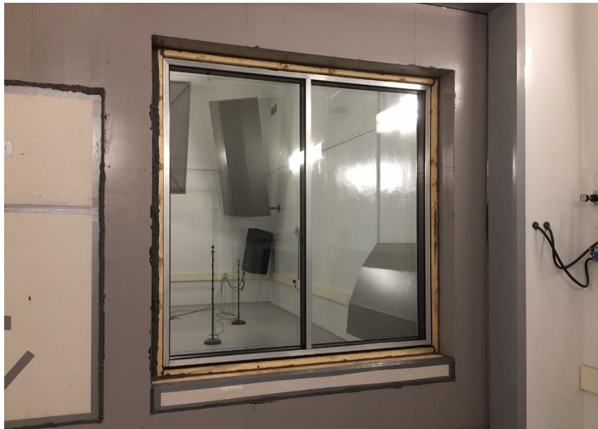
Source Room View of Installed Specimen
