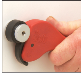
Tighten Base with Cat. No. ASW12 Adjustable Strap Wrench
