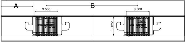
For two ply laminated glass with 1/4" Fully Tempered Glass and 1/16" interlayer maximum glass light height is 42":
