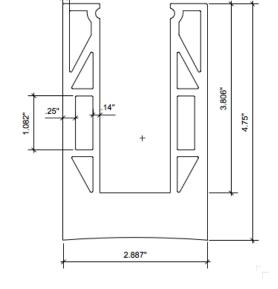
Allowable shear across cell - based on shear bending across cell legs allowing rotation at top
