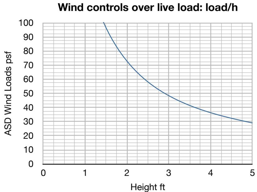
Glass thickness and light width must be adequate to support the imposed load.
