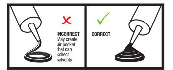
Do not apply mastics in a circle where an air pocket could collect solvents and possibly extract material that could be damaging to the mirror. The best way to apply Premier<sup>®</sup> Plus from a cartridge is to start from the center and let the mastic naturally expand out as it's being gunned.
