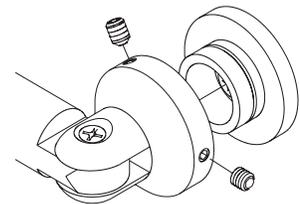
5. Place the Bracket at the center of the hole, with the slot in a vertical position. Drive the screw into the wall through the slot. Perform this operation on both top and bottom fittings.
