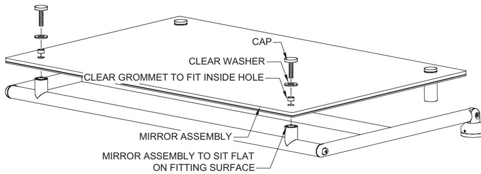
Place the clear grommet inside the hole and the clear washer over the hole. Add a couple drops of the provided Loctite Thread Locker to the last 1/3 of the threads of each Cap, and then screw the Caps into the frame.
